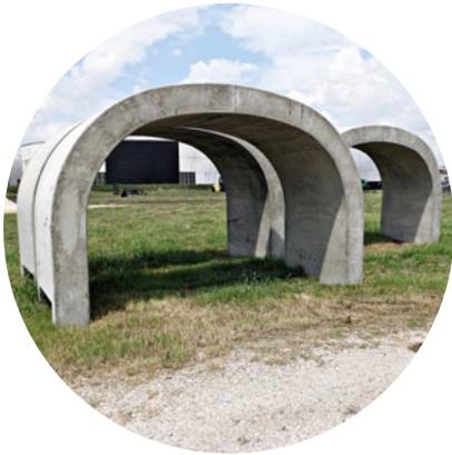
utilizing a poured-in-place concrete foundation combined with a precast concrete arched tunnel. The foundation is interlocked with the precast arched tunnel through a patented locking system that provides a way for the tunnel to be leveled. The process also generates a decrease in both schedule time and risk in construction.
