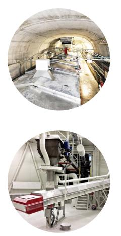
Reclaim systems play a significant role in explosion prevention. The systems shown above for wood pellet (top) and sugar (bottom) take special care to reduce the accumulation of combustible dust. produce heat, with either the drying effect or the hydrating effect causing self-heating. The dome's insulated nature also reduces heating and cooling of the walls and air inside, thus preventing condensation from forming and introducing moisture to the product.
